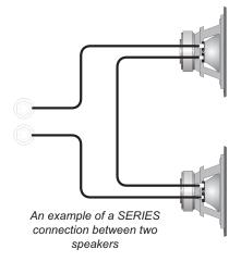
The total impedance of speakers in series is found by adding their impedances together. For example, two four ohm speakers in series is an eight ohm load. Series connections are easier on the amplifier than parallel connections as the total impedance is higher than driving a single speaker.
